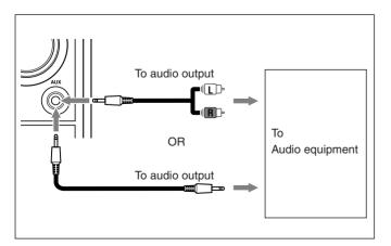
When the audio equipment has pin jacks for audio output: Be sure that the pin plugs of the audio cords are colored—white plugs and jacks are for left audio signals, and red ones for right audio signals.
